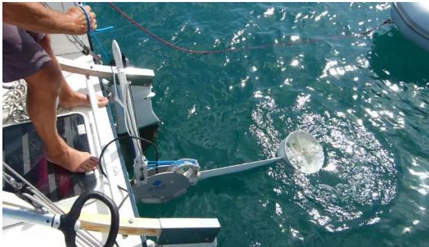
A person on a boat is pulling a blue rope. The hydrogenerator is being lifted out of the water, and a splash is visible. The boat is on the water, and a blue tarp is visible on the deck.                                                    |
